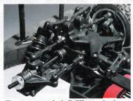
The outputs to the ball diffs are plastic, but use metal collars to make them hold together when you're hard on the throttle.
